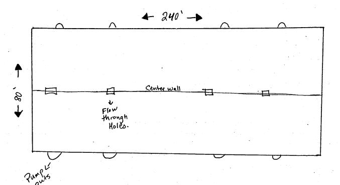
This Pit is 80' X240' and is 8' deep. the concrete is reinforced with rebar. There is a center support wall in the middle and there is 4 flow throughs at the bottom of the center wall. There are also 4 pump outs (PTO driven Certrificals) on each side of the building. The floor is 100% total slats.
